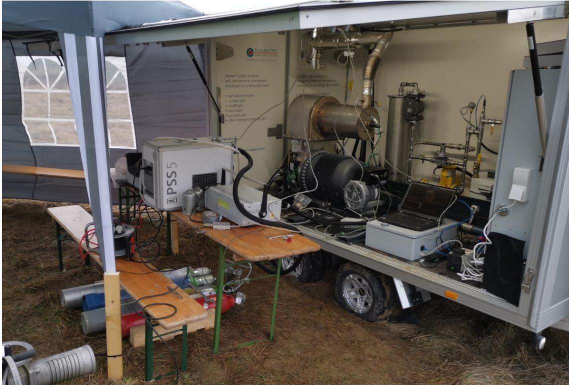
Figure 2: Measurement setup and Stirling cogeneration unit in the trailer.
