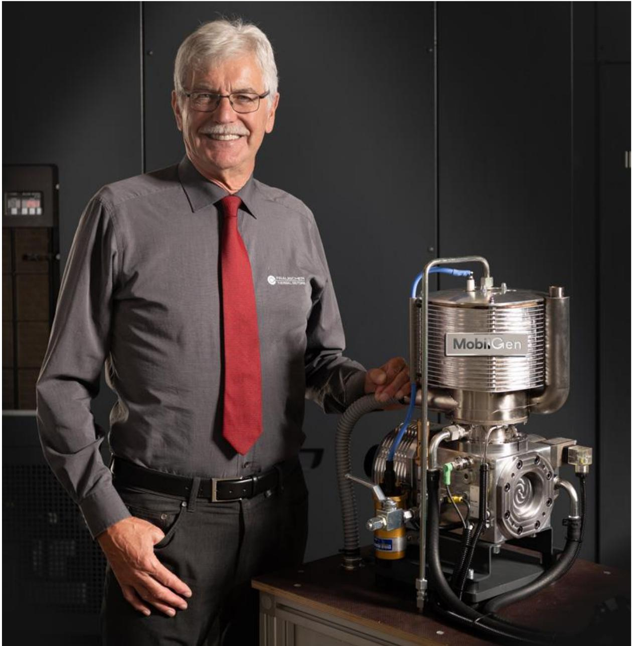
With the MobilGen™ G70, Ing. Josef Frauscher set a milestone in engine development. The new engine is planned to be used as an auxiliary power unit in trucks and supply electricity for the parking cooler and other consumers. (Use free of charge, image rights: Erwin Berghammer/Frauscher Thermal Motors)
